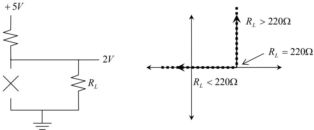
One gets  $V_{OUT} = 2V$  when  $R_L = 220$  ohms.
