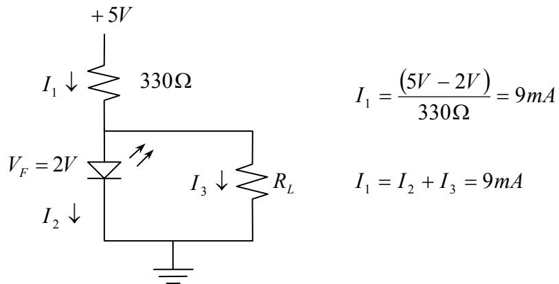
If  $R_L$  is such that  $V_{OUT} = 1V$ , there is no current flow through the diode. The diode conducts (turns on) when  $V_{OUT}$  hits  $R_L$ .
