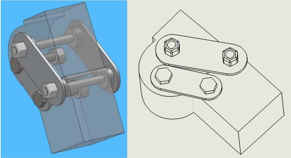
**Figure 10: Completed Assembly for Multiple Linkage Knee.** This assembly includes two high-density polyethylene blocks, two steel linkages, four bolts, and four lock nuts. The pieces to be manufactured are described in Figures 4,5,8,and 9. Note that two out of eight holes are countersunk, and that the design currently includes only three linkages. We will be investigating the effects of adding another linkage or damper in the same location this summer.
