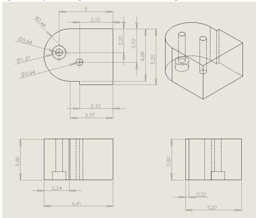
**Figure 8: Upper Portion of Multiple Linkage Knee.** Shown here is a three section view of our latter prototype's upper half. It is the same as that for the first prototype, except it contains two fewer countersunk holes.
