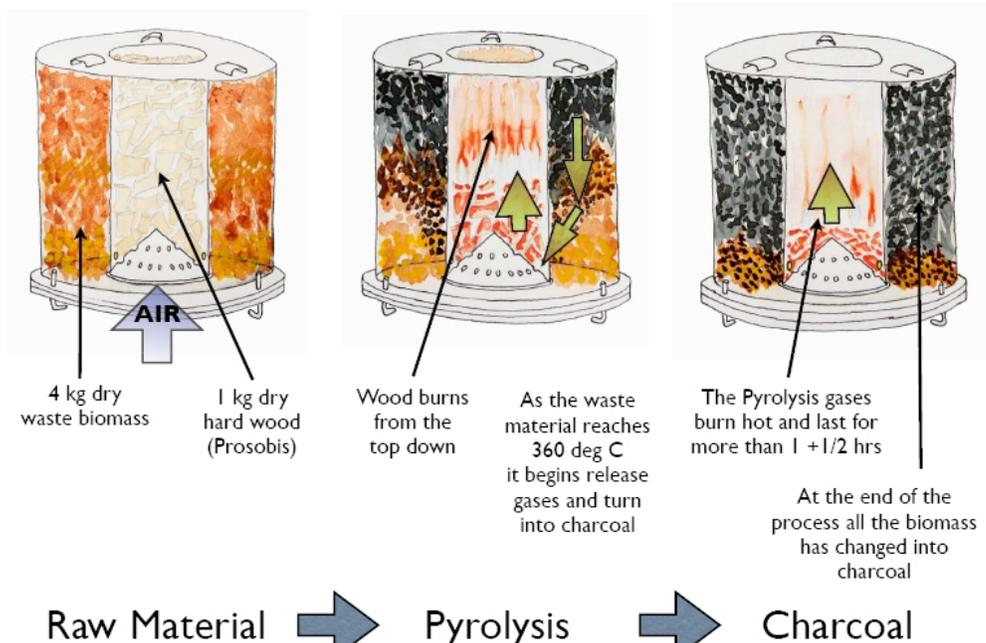
**Figure: Combustion Process for the Anila Stove**
