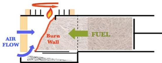
Figure 1. Schematic of a stove burn.
