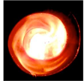
Figure 2b. Flames of the secondary burn traveling around the spiral.
