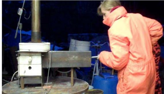
Figure 5. Plunging pine needles into the fuel shoot.
