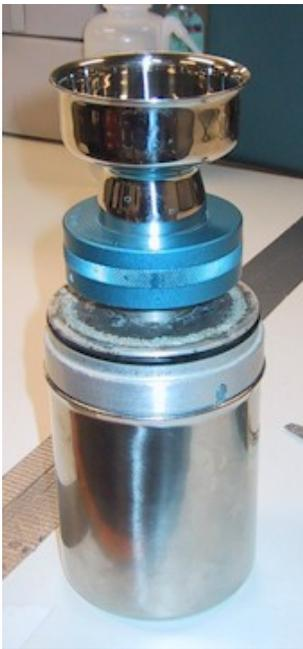
Figure 2: Millipore Field Apparatus
