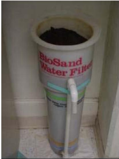
Figure 7. A prototype combined-filter
