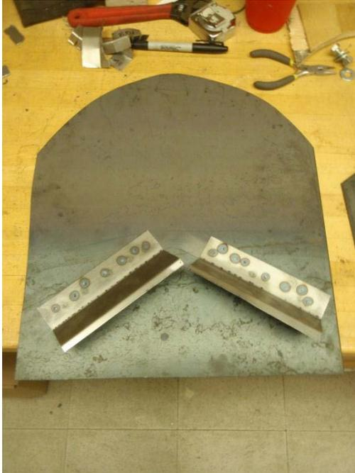
**Figure 4** - Plate with a spot-welded handle that sits 45 deg. to the plate, with a semi-circular edge.
