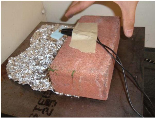
**Figure 6** - Thermopile setup mounted to brick and set over very crinkled foil; entire setup on top of hotplate
