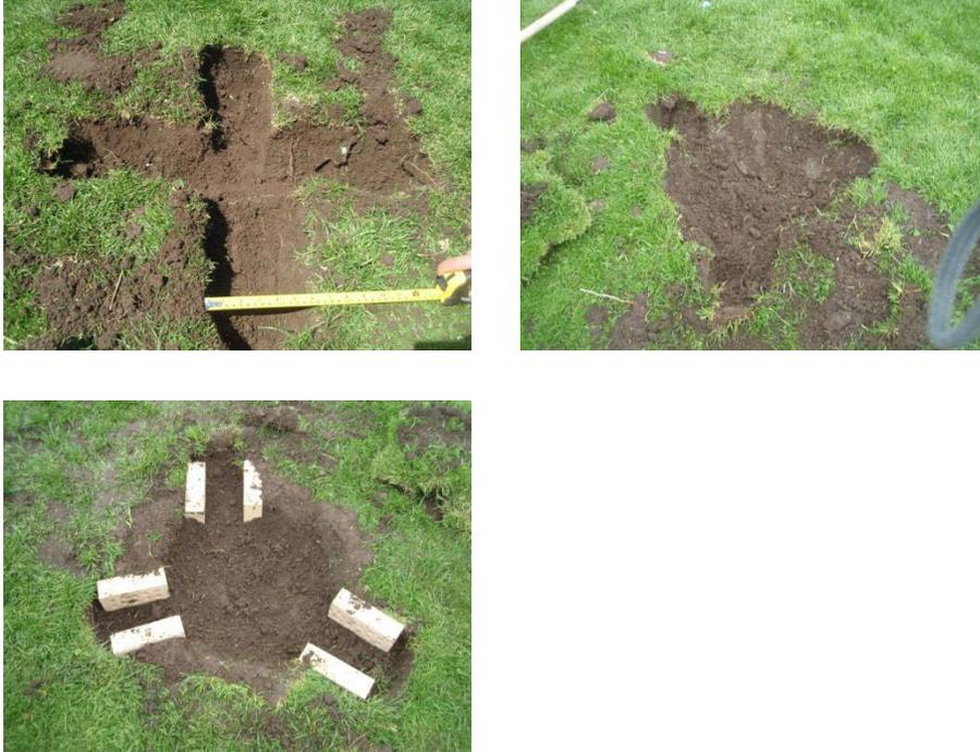
**Figure 3** - Counter-clockwise from top right: Circular dugout with 3 dirt channels, Cross-shaped dugout, and circular dugout with 3 brick-lined channels
