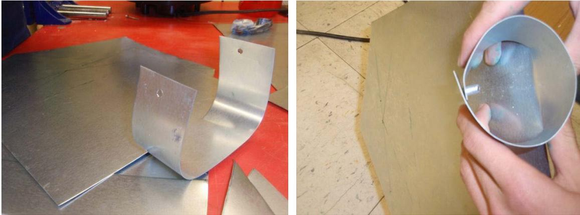
**Figure 11** – Bending and riveting the sheet metal to create the handle
