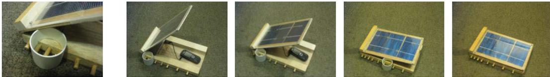
*Fig. 6: Notch and Wedge Adjustment System*
