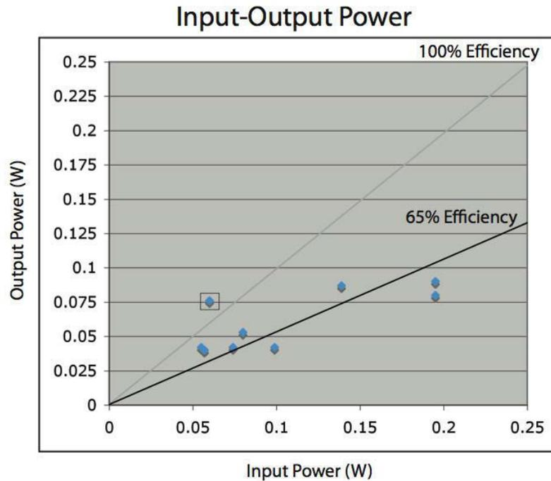
*Fig. 9: Input-Output Data Graph. Figure above shows the input and output data for the solar cell phone charger. Note the linear fit on the input over output data.*
