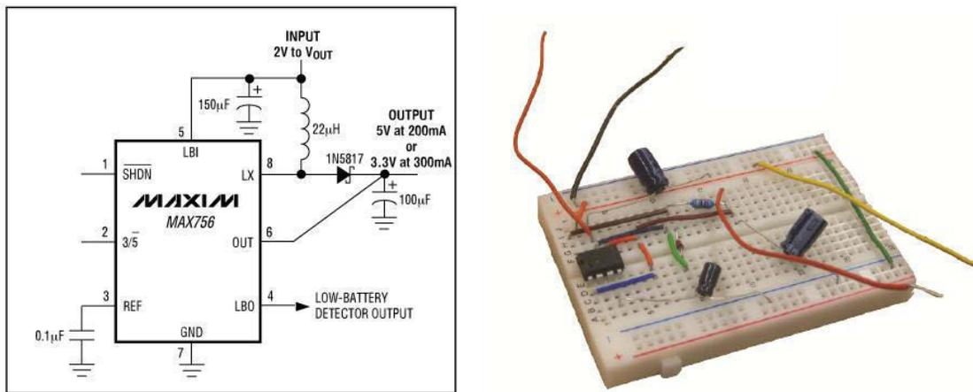
*Fig. 5: Circuit Diagram and Final Circuit using this Setup*
