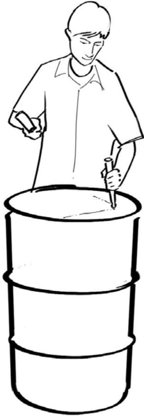
Cut a large opening for filling the kiln with the material you want to carbonize.
