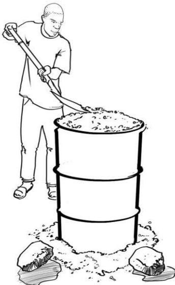
Seal the bottom edges and the top of the drum with sand or dirt to prevent oxygen from entering. Wait at least 2 hours before opening.
