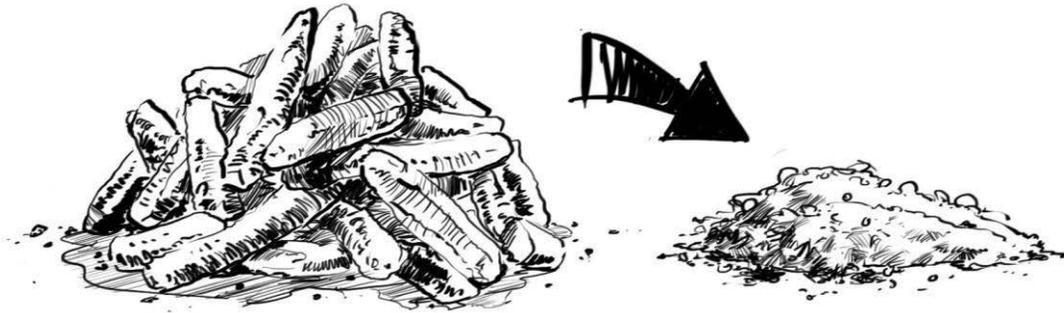
There are many ways to crush charcoal. Adding water while crushing helps to prevent dust from spreading around.
