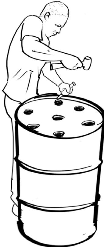
Cut several holes in the bottom of the drum. These holes allow air to flow through the drum while burning, which results in a hotter fire and produces better charcoal.
