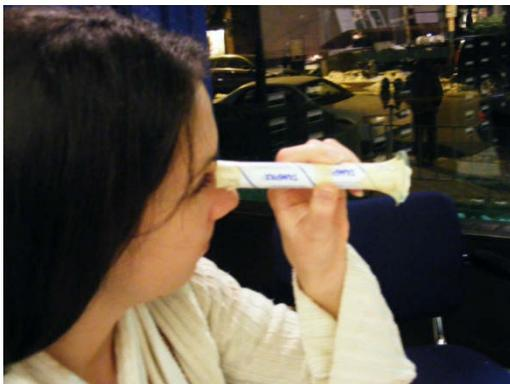
LJ and I begin to make a telescope. We have a 6 inch, 11/16 inch in diameter tube. We attach the very thin concave lens to one end of the tube. We attach the plano-convex lens to the other end (convex shape is on the outside). How does this work? We create a set up to measure how much we can see at different distances. How much does what we see increase or
