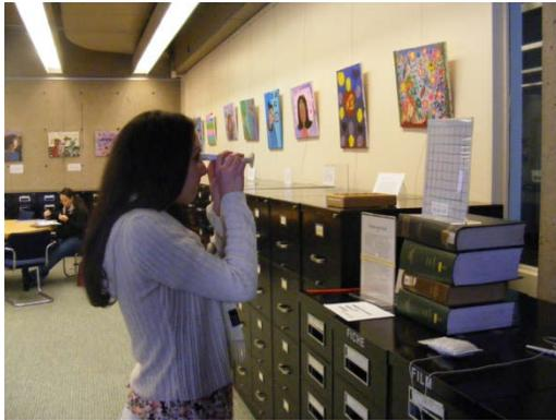
the squares as we could get, we moved back until we could see 2 x 2, then 4 x 4, then 6 x 6, and 8 x 8 squares. Each time we recorded the distance. We repeated this twice, once with Leigh and once with me. We took the average distance between our two measurements. LJ then used a similar tube with no lens to see what she could see. The
