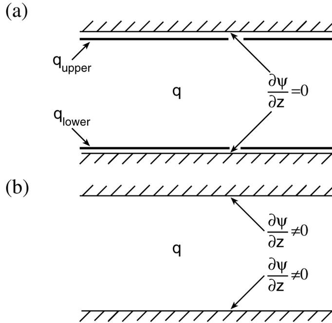
Figure 5: In (a)  $\hat{q} = q + q_{upper} + q_{lower}$  is inverted with homogeneous boundary conditions  $\frac{\partial \psi}{\partial z} = 0$  where  $q_{upper}$ ,  $q_{lower}$  are PV  $\delta$ -function sheets adjacent to the boundary but just interior to the fluid. In (b)  $q$  is inverted with inhomogeneous boundary conditions  $\frac{\partial \psi}{\partial z} \neq 0$ . If the sheets are chosen to have strengths given by eq(23), the interior solutions are identical.
