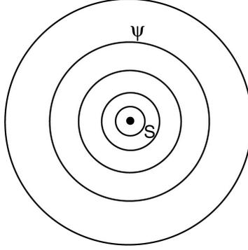
Figure 2: A point vortex of strength ‘ $s$ ’ induces a circulation  $\Psi$  given by eq., if  $f$ ,  $N = \text{constant}$ , eq.(21).
