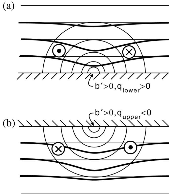
Figure 6: (a) warm lower boundary induces cyclonic circulation aloft (b) warm upper boundary induces anticyclonic circulation below.
