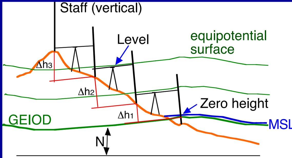
Orthometric height of hill is  $\Delta h_1 + \Delta h_2 + \Delta h_3$
