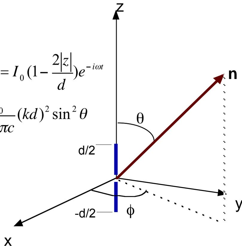
P is the radiated power from the antenna, with current  $I_0$  center fed into antenna
