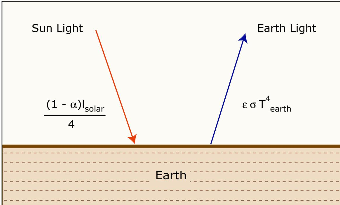
$$F_{\text{out}} = 4\pi r_{\text{earth}}^2 \epsilon \sigma T_{\text{earth}}^4$$
