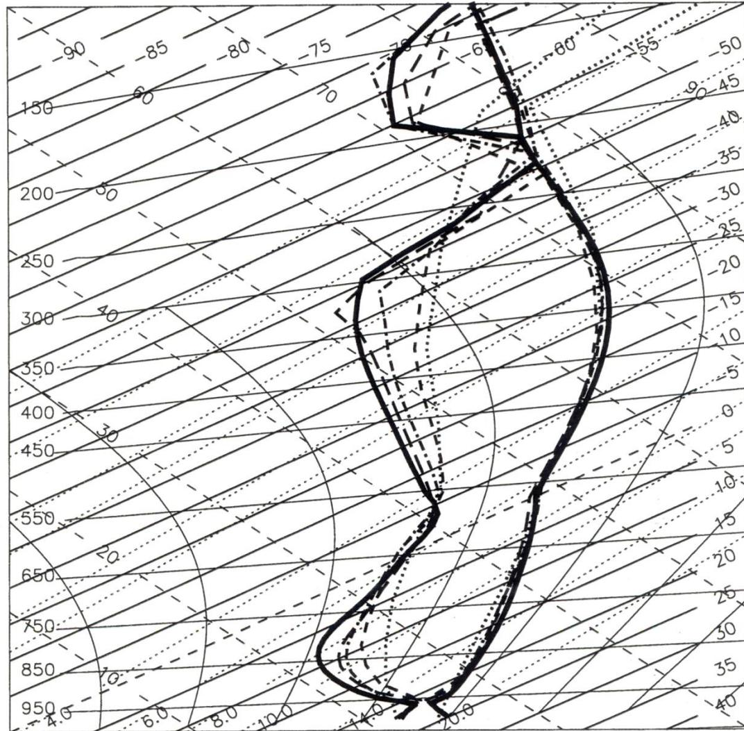
Figure 8. Tephigram plotting equilibrium temperature (lines on right) and moisture (lines on left) for the Emanuel model using 10 vertical layers (dotted lines), 20 vertical layers (dashed lines), 30 vertical layers (dot-dash lines), 40 vertical layers (long dash lines), 50 vertical layers (solid lines), in addition to the 10 layers placed above 100 hPa.
