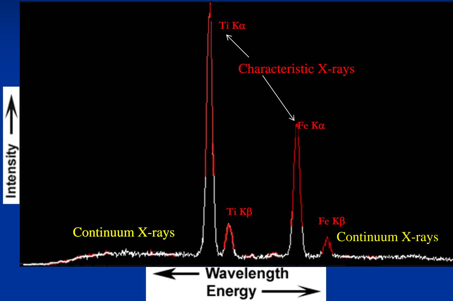
*Continuum X-rays are generated by deceleration of beam electrons in the Coulombic field of outer shells of target atoms. Maximum energy = electron beam energy*
