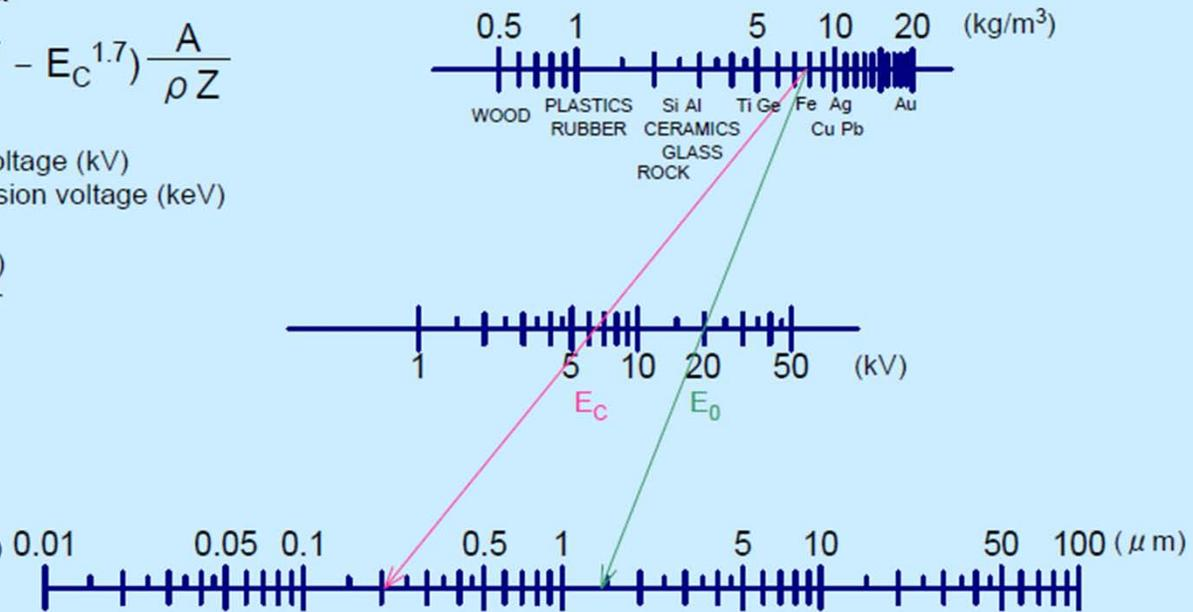
Analytical area of iron in 20kV  $\cong 1.5 - 0.2 = 1.3 (\mu\text{m})$
