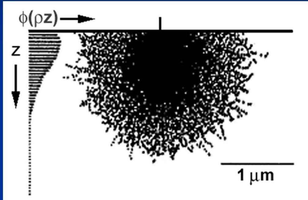
$\phi(\Delta\rho z)$  = intensity from a freestanding layer of thickness 'z'
