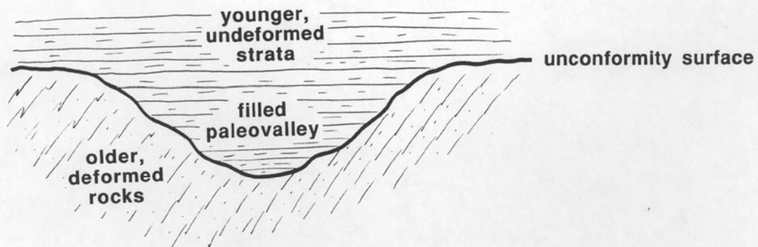
Figure 8-11. A buttress unconformity.
