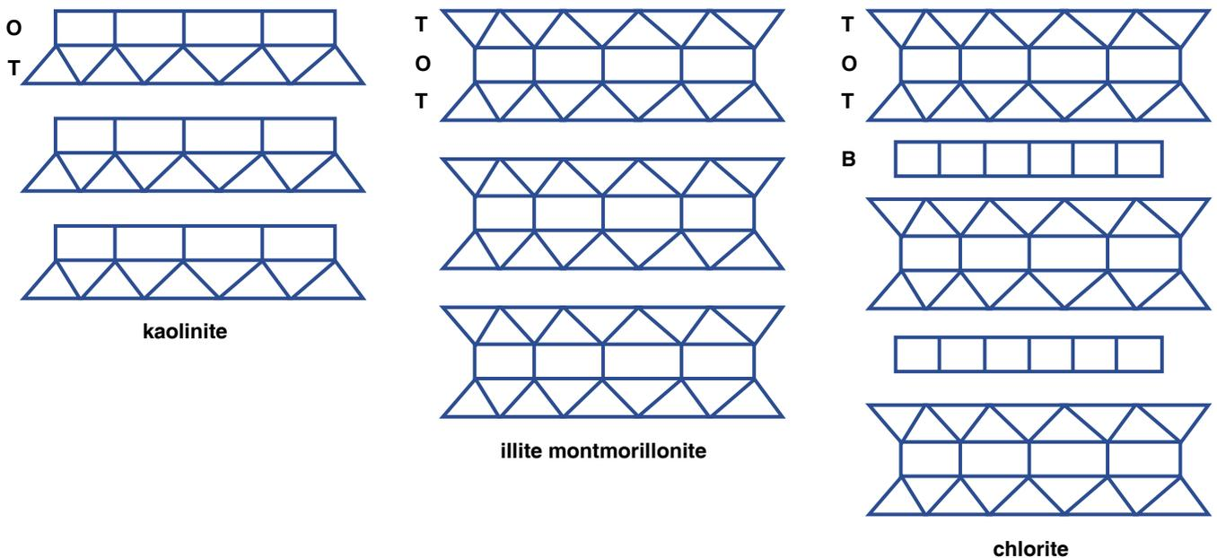
Figure 4-13: Sketches of the structural organization of clay minerals
