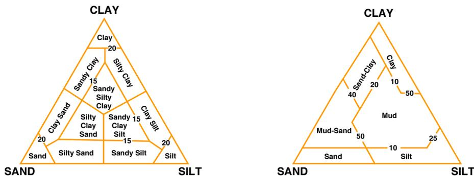
Figure 4-1: Two classifications of mixtures of sand, silt, and clay
