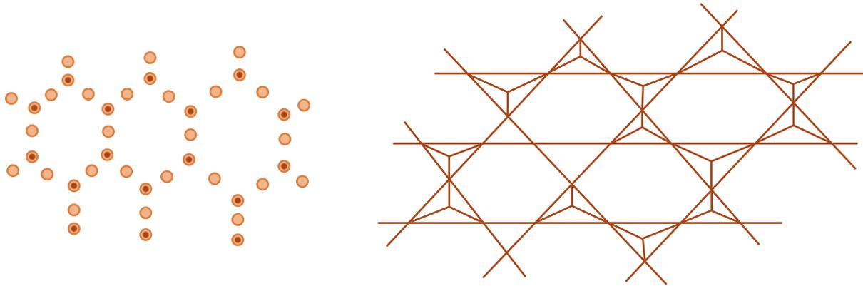
Figure 4-10: Diagrammatic representations of the arrangement of silica tetrahedra in the tetrahedral sheet of clay-mineral structures
