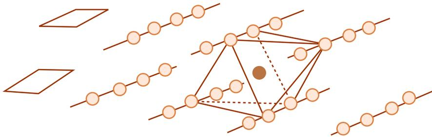
Figure 4-8: Sketch of the arrangement of atoms in the octahedral sheet of clay-mineral structures
