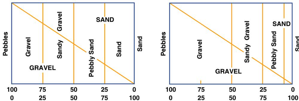
Figure 4-2: Two classifications of mixtures of sand and gravel
