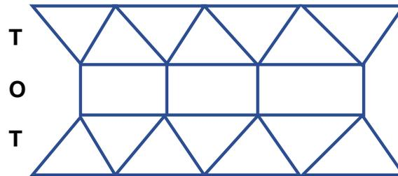
Figure 4-12: Sketch of the combination of octahedral in three-layer clay-mineral structures and tetrahedral sheets
