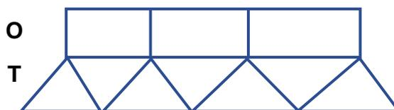
Figure 4-11: Sketch of the combination of octahedral and tetrahedral sheets in two-layer day-mineral structures
