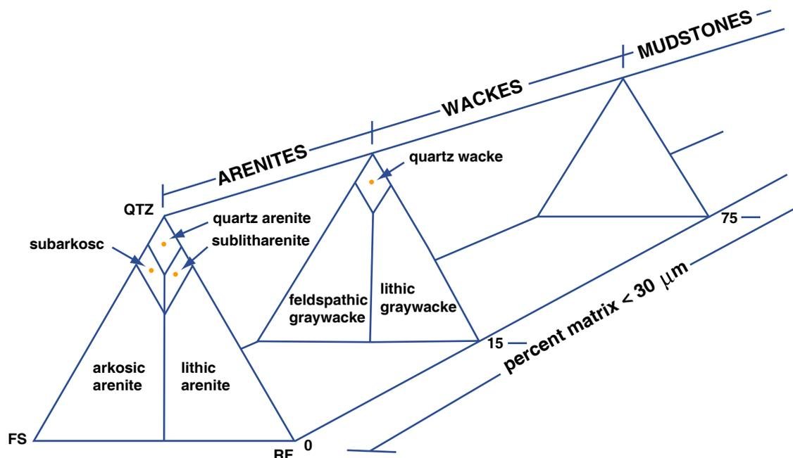
Figure 4-3: The Pettijohn/Potter/Siever classification, of sandstones
