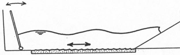
**Figure 2-58** Oscillatory flow in a wave tank
