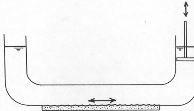
**Figure 2-59** Oscillatory flow in a closed duct
