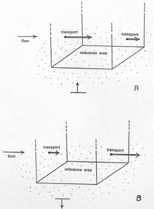
**Figure 2-68** Sediment transport over the reference area. A: Sediment is being added to the flow from the bed somehow, so there's net erosion. B: Sediment is being added to the bed from the flow somehow, so there's net deposition.
