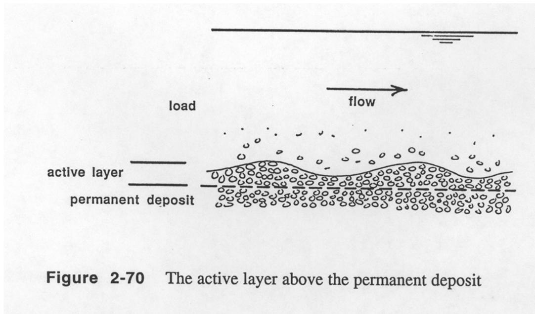
**Figure 2-70** The active layer above the permanent deposit
