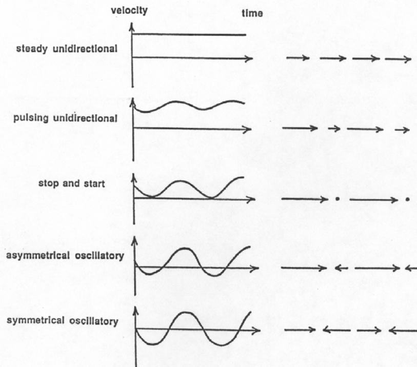
**Figure 2-40** Spectrum of kinds of combinations of unidirectional and oscillatory flow components in combined flow
