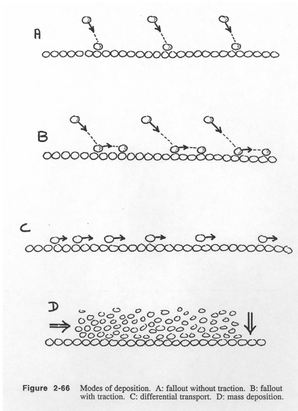
Figure 2-66 Modes of deposition. A: fallout without traction. B: fallout with traction. C: differential transport. D: mass deposition.
