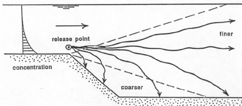
**Figure 2-57** Some fraction of the transported grains are carried beyond the crest above the separation surface, to settle through the complicated turbulent flow field in the wake of the ripple and land at various points
