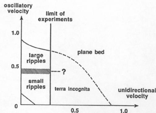
**Figure 2-65** Extrapolation of the combined-flow bed-configuration graph of Figure 2-64 to greater unidirectional velocities
