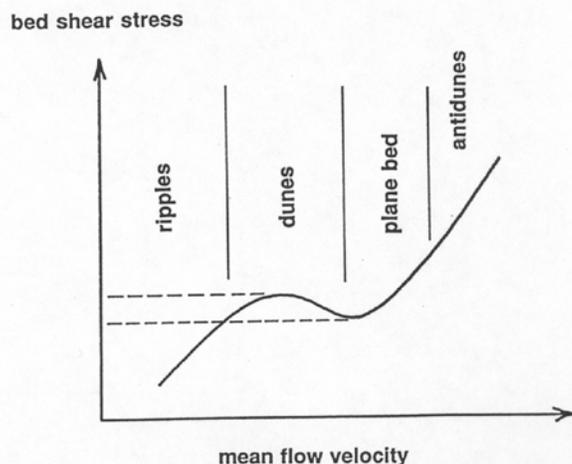
**Figure 2-45** Cartoon graph of bed shear stress against mean flow velocity, showing the dip in the curve caused by the decrease in flow resistance in the transition from dunes to plane bed
