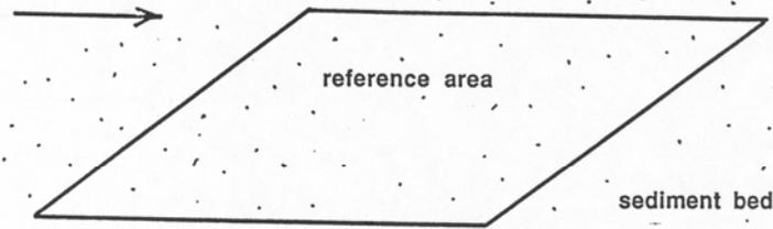
**Figure 2-67** A small rectangular reference area on the sediment bed beneath a flow that's transporting sediment over the bed
