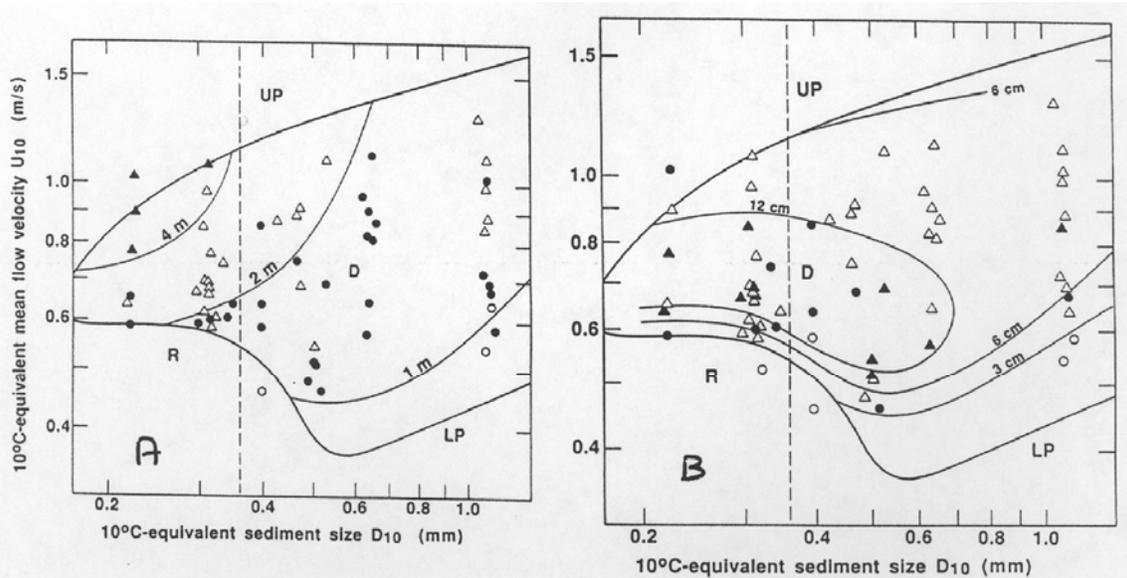
**Figure 2-52** Crude contours of dune spacing (A) and dune height (B) in a velocity-size section. Symbols as in Figure 2-52.
