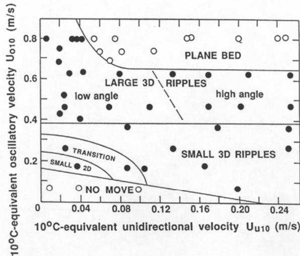
**Figure 2-64** Combined-flow bed-configurations in a graph of oscillatory velocity component against unidirectional velocity component for a sand size of about 0.1 mm and an oscillation period of about 9 s. Solid circles, combined-flow ripples; open circles, sediment movement on a plane bed (above the ripple field) or no sediment movement on a plane bed (below the ripple field).
