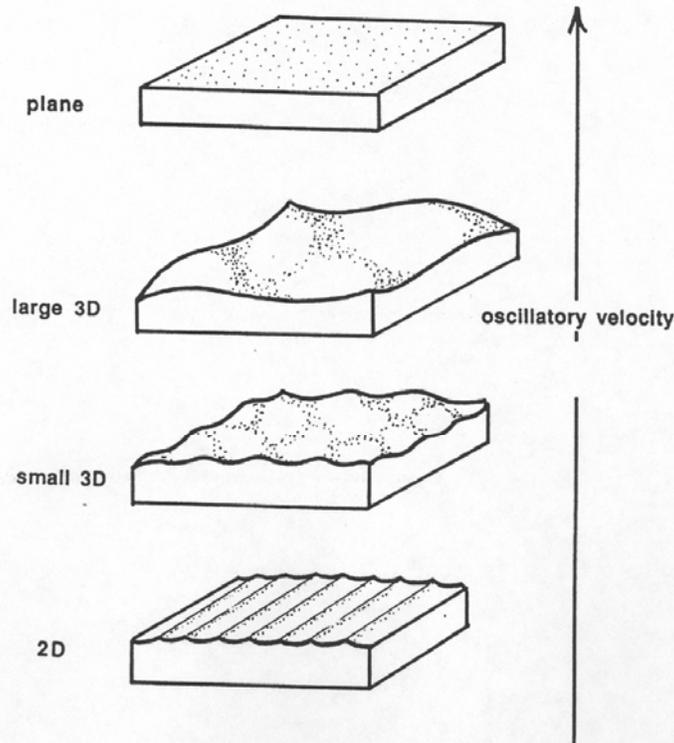
**Figure 2-61** Sequence of oscillatory-flow bed configurations with increasing flow strength at a moderate to long oscillation period
