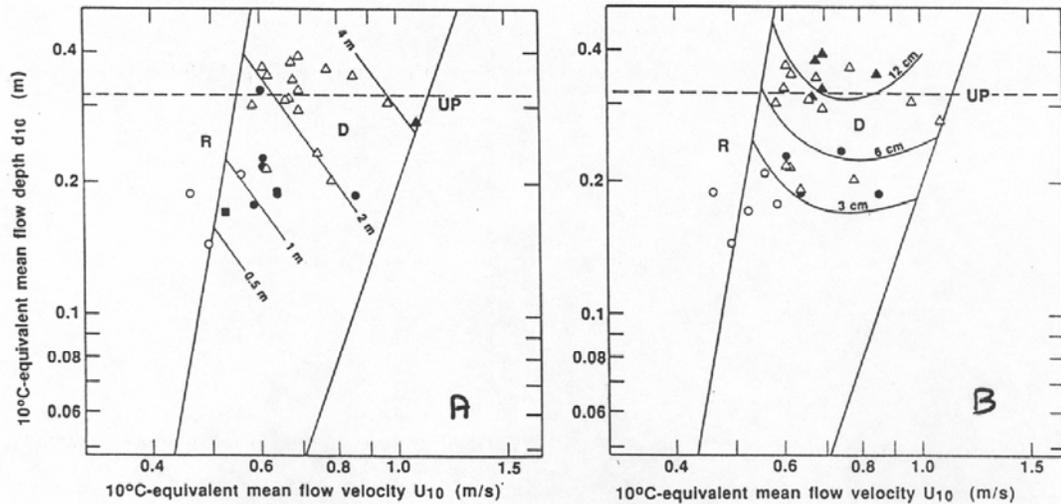
**Figure 2-51** Crude contours of dune spacing (A) and dune height (B) in a depth-velocity section. Symbols for dune spacing: solid squares, <0.5 m; open circles, 0.5-1 m; solid circles, 1-2 m; open triangles, 2-4 m; solid triangles, >4 m. Symbols for dune height: open circles, <3 cm; solid circles, 3-6 cm; open triangles, 6-12 cm; solid triangles, >12 cm.
