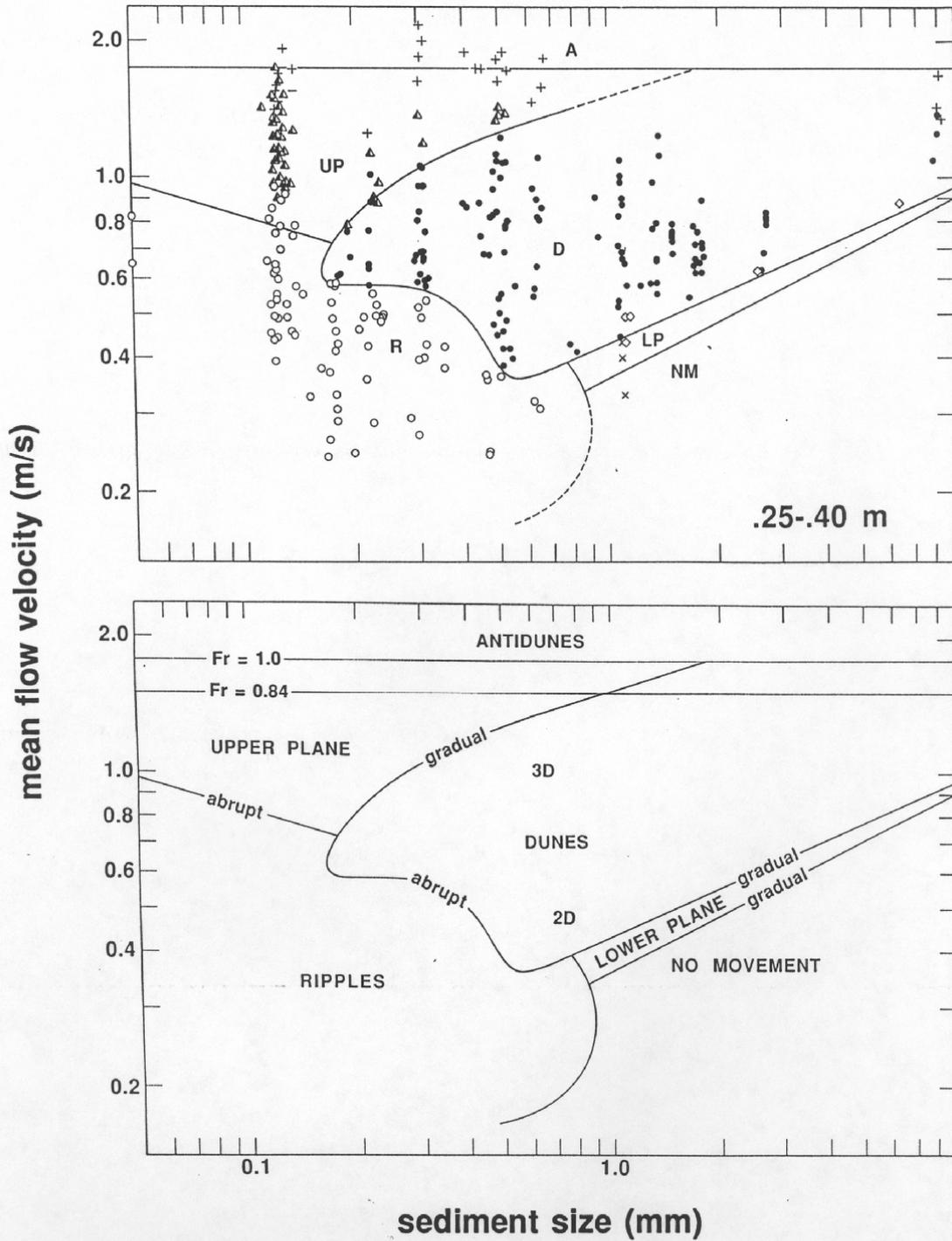
**Figure 2-48** Velocity-size section for a flow depth of 0.25-0.40 m through the depth-velocity-size diagram for bed phases in unidirectional flow. Symbols are the same as in Figure 2-47.
