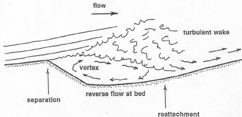
**Figure 2-54** More cartoonlike version of Figure 2-53 showing the general structure of separated flow over a ripple or a dune
