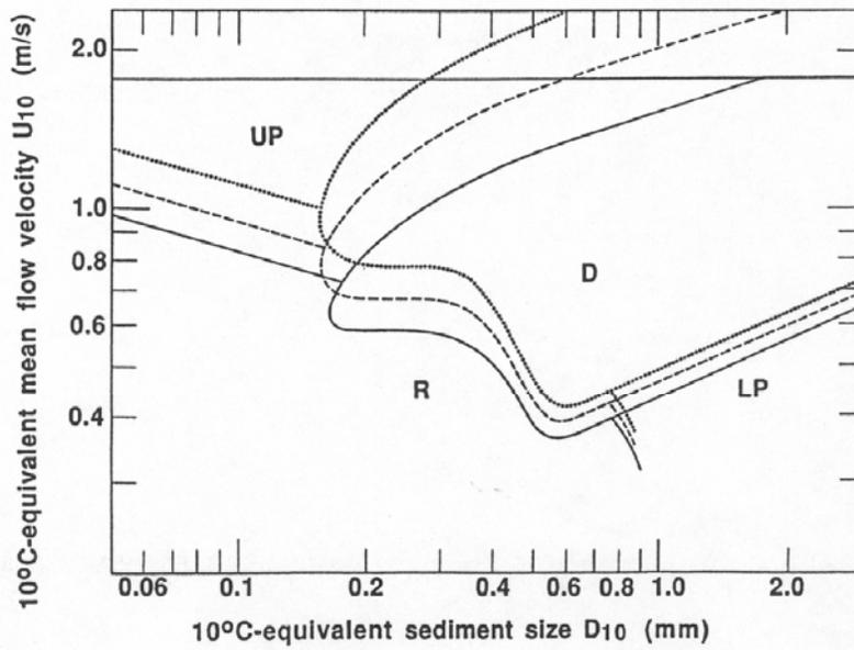
**Figure 2-49** Schematic velocity-size sections, superimposed on the same plot, for flow depths of 0.3 m, 1 m, and 3 m
