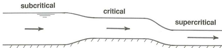
Figure 5-12. The behavior of the flow over a rise and then a fall of the channel bottom, when an approaching subcritical flow is forced to the critical condition by raising the step by a sufficiently large increment.
