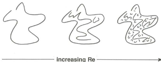
Figure 4-23. Increase in the range of eddy scales as a function of mean-flow Reynolds number.
