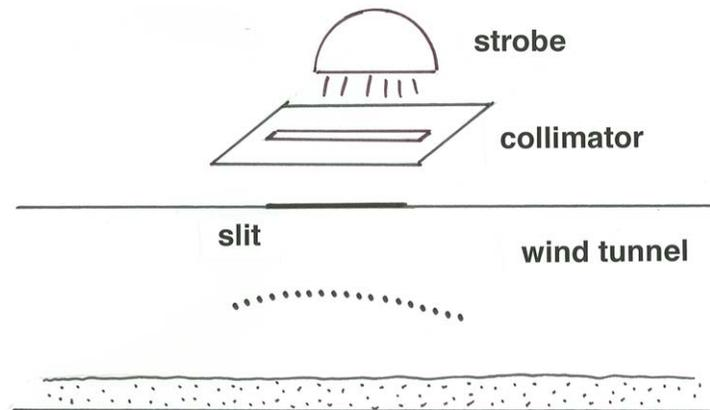
Figure 11-3. A lighting arrangement to see saltation trajectories.
