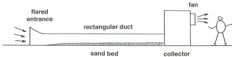
Figure 11-2. A simple but effective wind tunnel.
