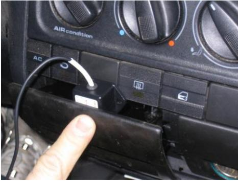
Figure 7: The accelerator was placed in the front, middle console of the car.
