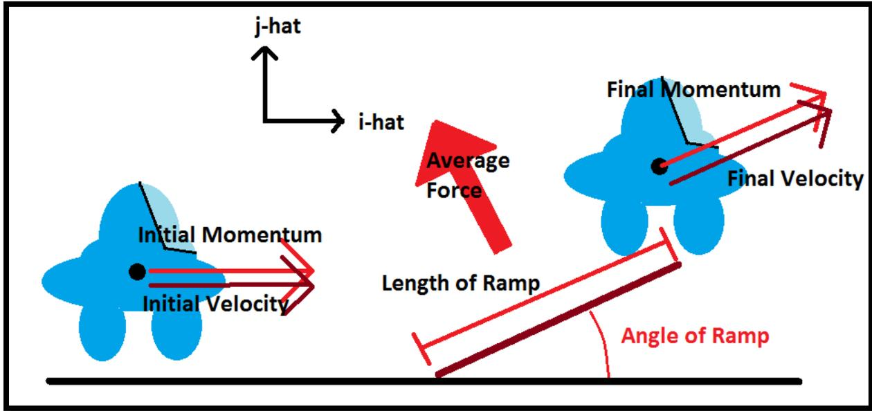
Figure 17: This is a simple sketch on which the model is based. Note the time to clear the ramp is simply the length of the ramp divided by the initial speed.
