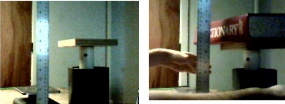
Figures 13-14: These are two pictures of the testing setup for the dashpot. Weights (books) were added to the dashpot and the rate of compression was measured using a video recorder on a laptop. The ruler measured the distance dropped and the video footage measured the time elapsed. The terminal velocity of the dashpot was measured in this way. Shown in the left picture is the scale that was used to measure the weight of the books.
