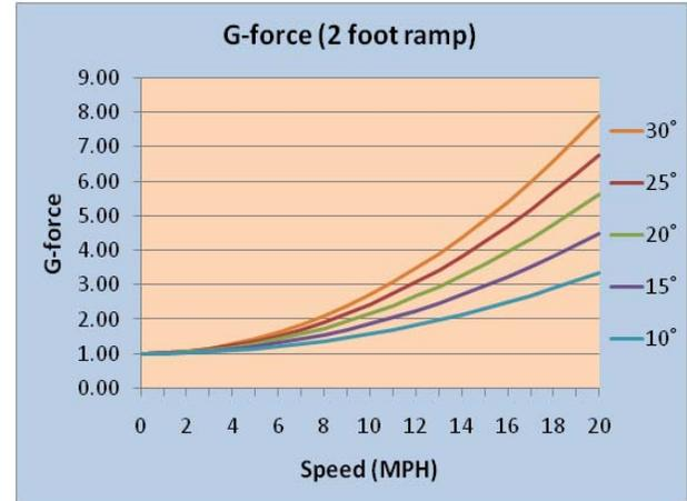
Figures 18 and 19: Graphs of the average g-forces applied to a vehicle riding over 1.5 and 2 foot angled ramps. Notice the changes in scale that reflect change in the magnitude of the average acceleration.
