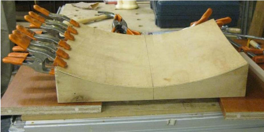
Figure 5: Bendable plywood can be easily shaped into a parabolic cylindrical surface. The pictures shows the gluing process of attaching the supporting beams that prevent the bendable plywood from bending in any way other than in the parabolic cylindrical shape
