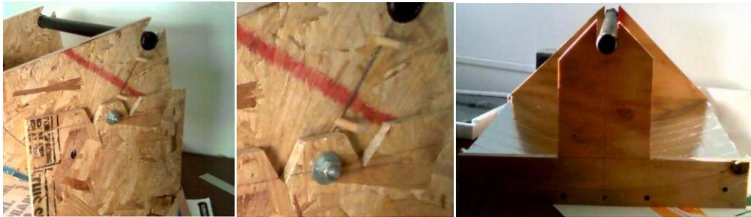
Figure 3: First two pictures are initial dowel aligning device. The third picture shows the improved design. Parallel rays do not cast a shadow from the side piece when the device is parallel to incoming rays.
