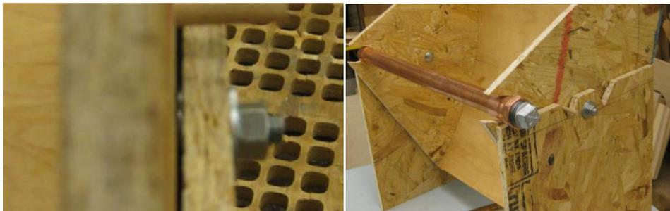
Figure 4: The new angling technique is shown from first the front view and then obliquely angled from the side. The central washer that constitutes the gap in between the wood pieces in the first picture is used to make up for the protruding heads of the screws used to attach the braces to the side piece (not shown). The bolts are pressed into the wood. We used clamps to do this. This keeps the bolt from turning. Then the nut can be tightened sufficiently using just one hand.
