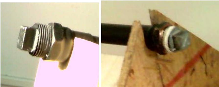
Figure 6: White pipe tape was used to help seal the plug. The first pictures shows the threads without pipe tape and the second picture shows the threads with the pipe tape. The pipe tape is intended to fill in the spaces between the threads.
