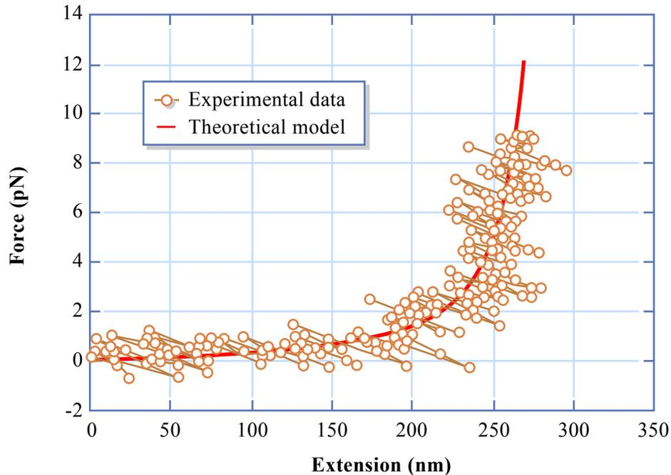
The force-extension curve for stretching a single type II collagen molecule. The data were fitted to Marko-Siggia entropic elasticity model. The molecule length and persistence length of this sample is 300 and 7.6 nm, respectively.
