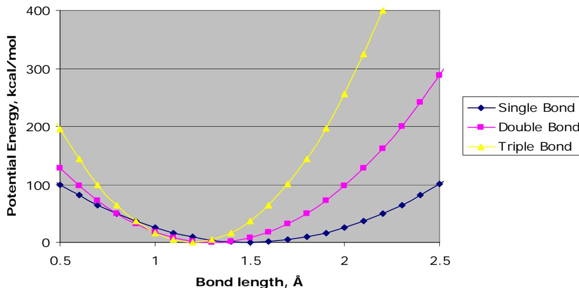
$$V_{\text{bond}} = K_b (b - b_0)^2$$
