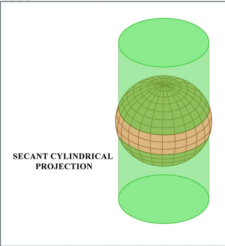
Earth intersects the cylinder on two small circles. All points along both circles have no scale distortion.
