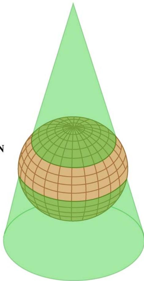
Earth intersects the cone at two circles. all points along both circles have no scale distortion.
