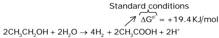
$\Delta G_{\text{reaction}}$  depends on H<sub>2</sub> partial pressure
