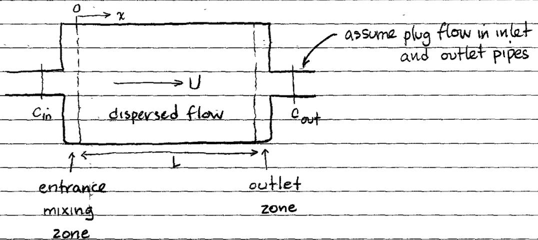
For the configuration as sketched small inlet and outlet pipes relative to tank cross section, we can assume plug flow in the pipes (i.e. dispersion is negligible).
