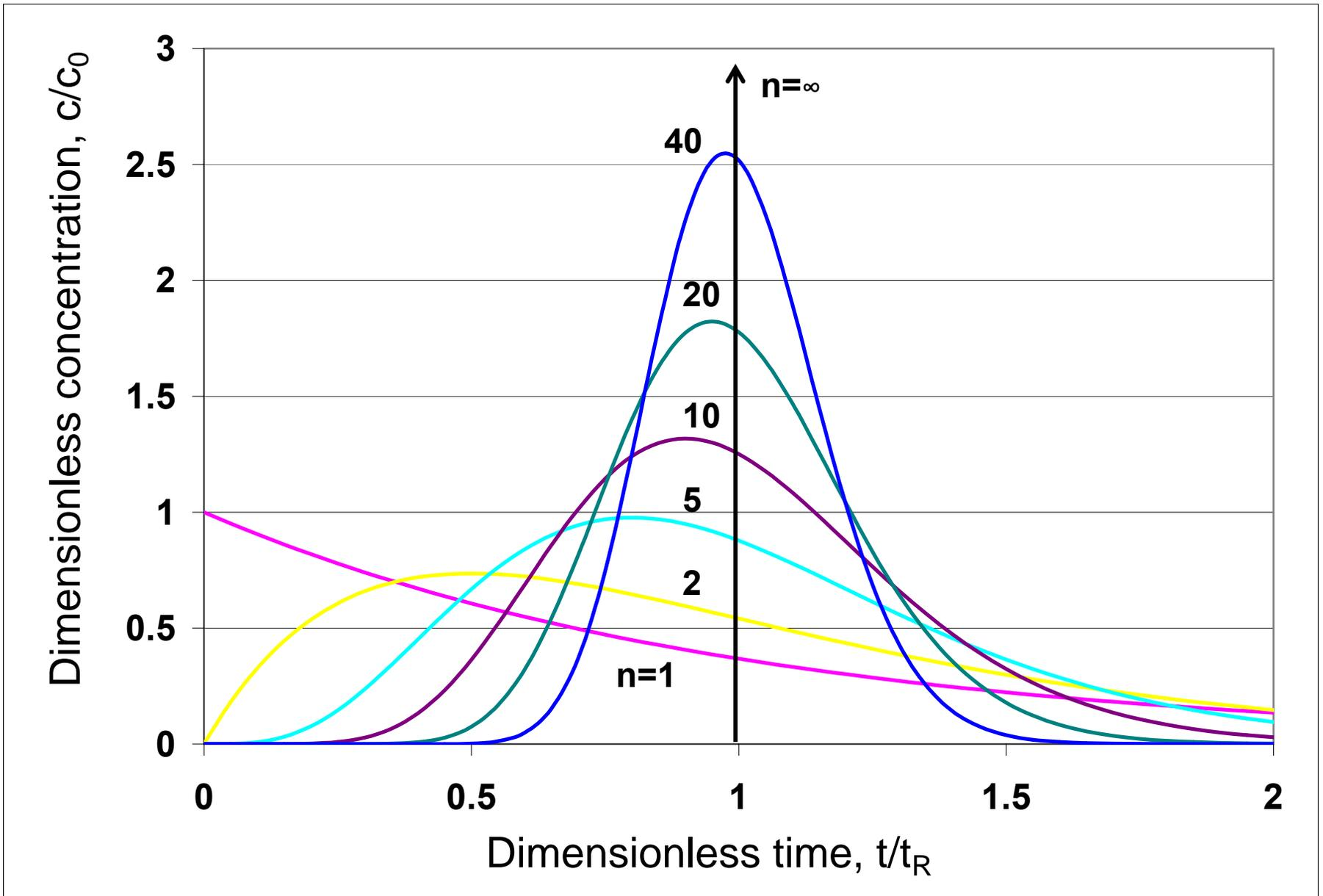
Tanks in series behave like dispersed flow reactor - see figure on page 12
