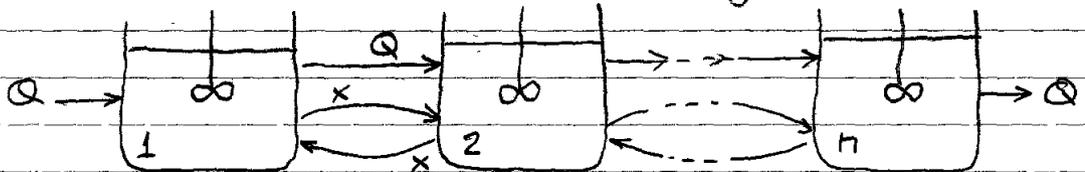
Exchange flow creates the effect of additional mixing and in the limit of infinite exchange flow makes a tanks-in-series reactor look like a FMT
