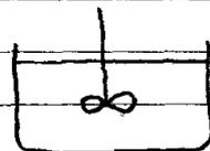
Ideal CFSTR has uniform concentration within its confines - influent is mixed instantaneously and completely
