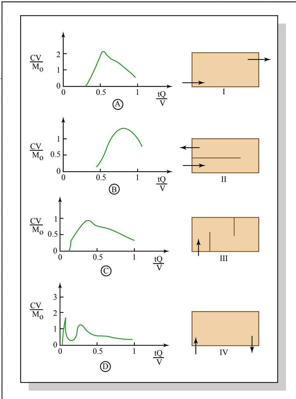
Can you place the UIR (A-D) with the schematic cooling pond (I-IV)?
