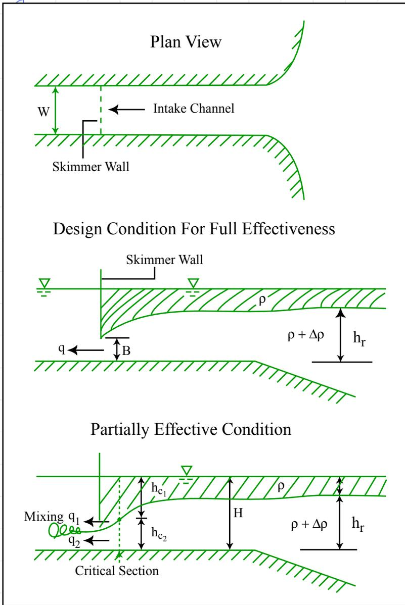
Selective withdrawal of water from density stratified tank or reservoir
