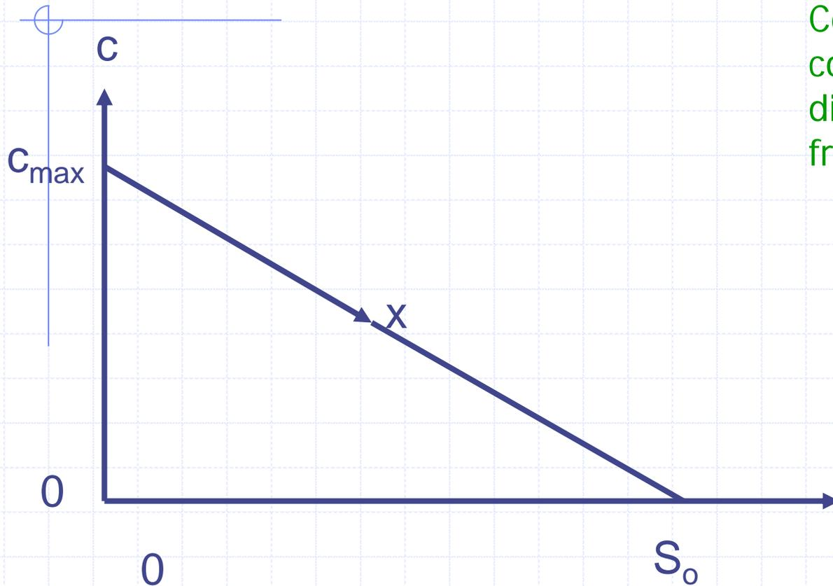
Concentration of conservative contaminant discharged at head (using freshness as tracer)
