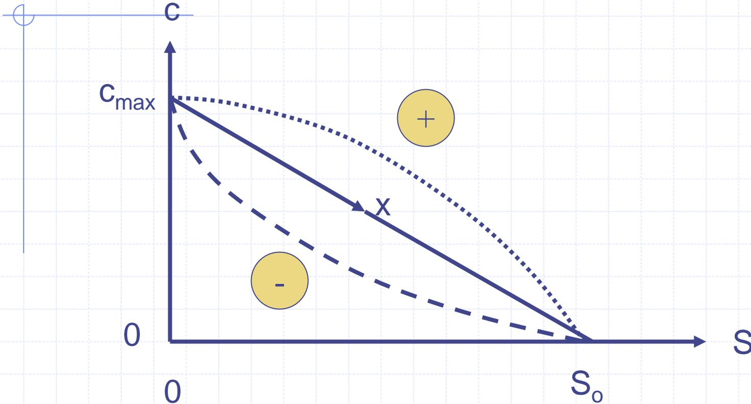
Note that conservative mixing curve is only linear if conditions are steady and there is a single source
