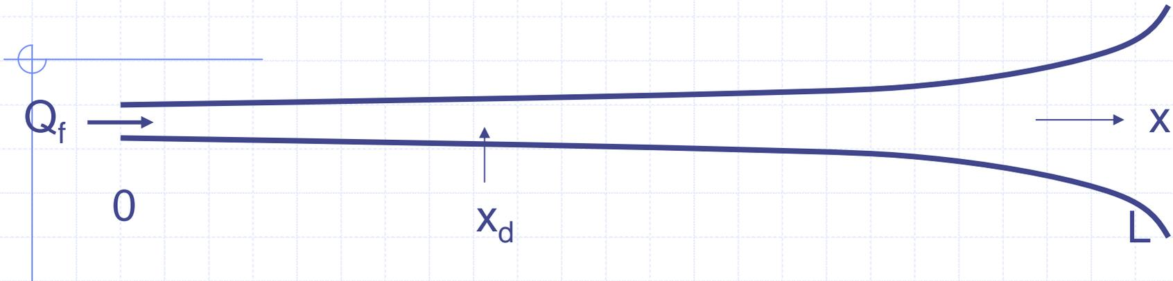
Use measured salinity distribution  $S(x)$  resulting from river discharge  $Q_f$  entering at head ( $x=0$ ) to infer concentration distribution  $c(x)$  of mass entering continuously at downstream location  $x_d$ .
