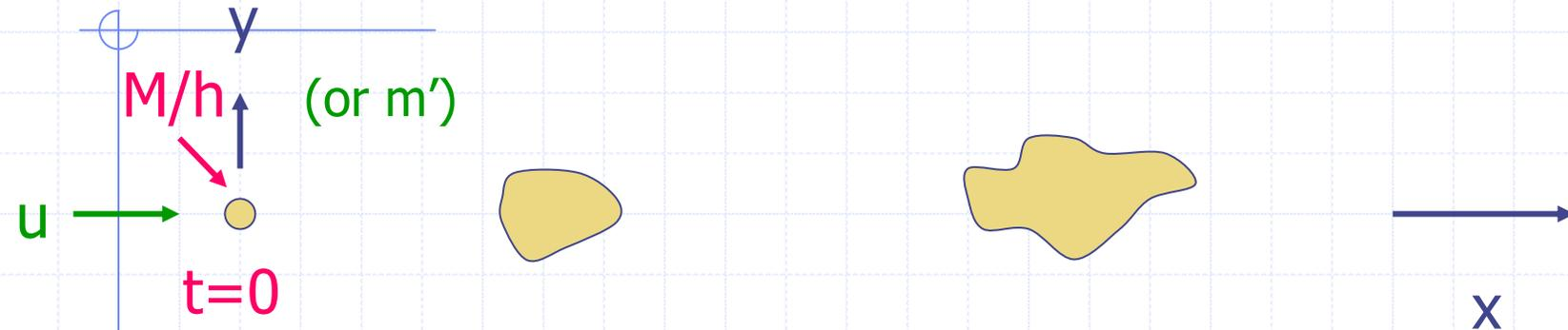
$$\frac{\partial c}{\partial t} + u \frac{\partial c}{\partial x} = E_x \frac{\partial^2 c}{\partial x^2} + E_y \frac{\partial^2 c}{\partial y^2} - kc$$
