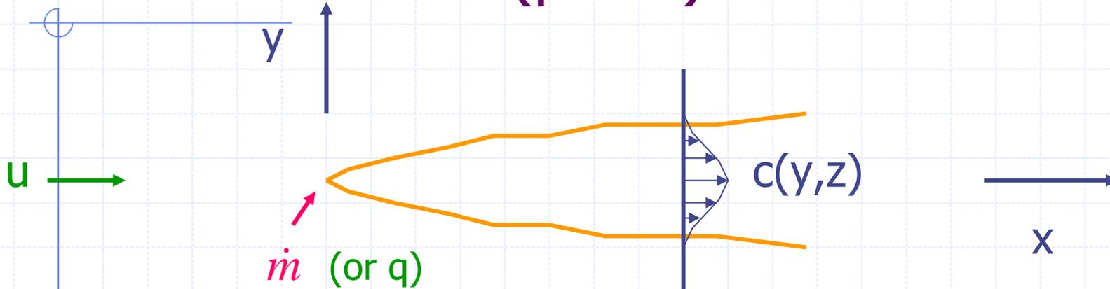
$$u \frac{\partial c}{\partial x} = E_x \frac{\partial^2 c}{\partial x^2} + E_y \frac{\partial^2 c}{\partial y^2} + E_z \frac{\partial^2 c}{\partial z^2} - kc$$
