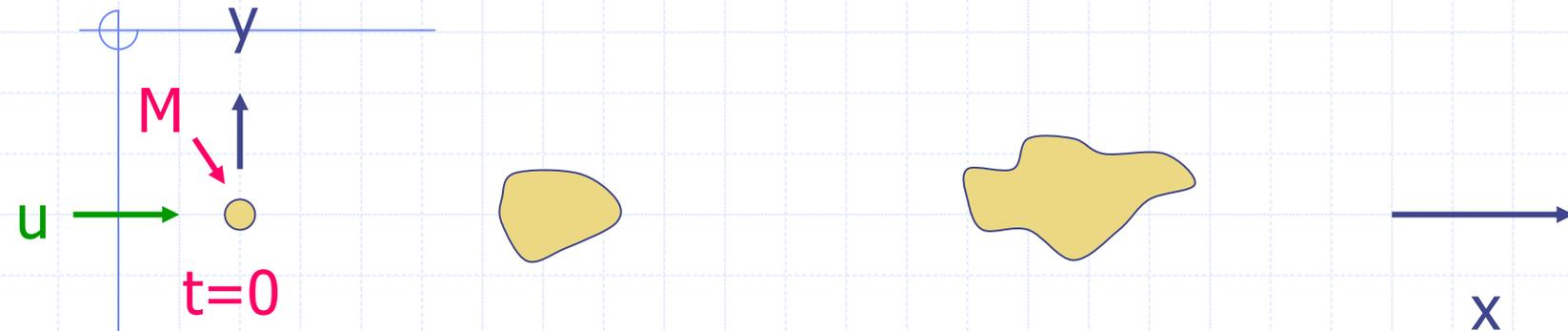
$$\frac{\partial c}{\partial t} + u \frac{\partial c}{\partial x} = E_x \frac{\partial^2 c}{\partial x^2} + E_y \frac{\partial^2 c}{\partial y^2} + E_z \frac{\partial^2 c}{\partial z^2} - kc$$
