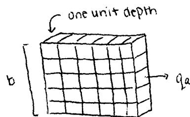
$bq_a$  calculates discharge through a cross-sectional area of  $b \times 1$  unit
