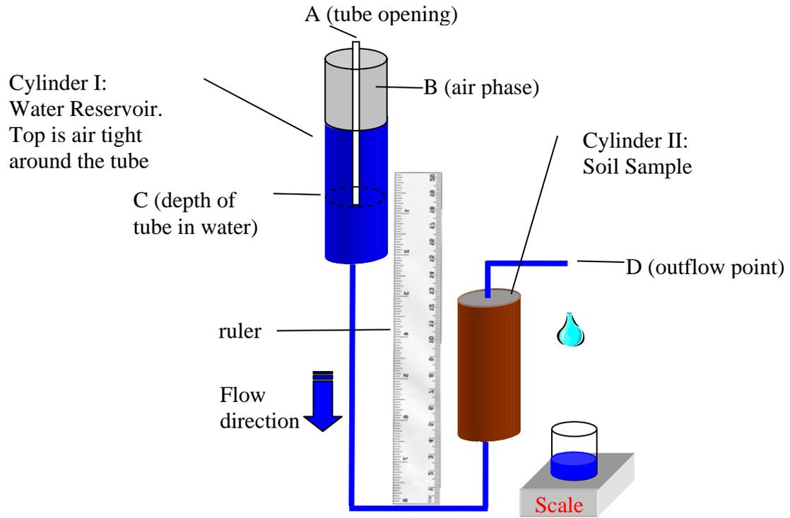
There has been a lot of confusion about how this system maintains a constant head without water flowing into Cylinder I. An explanation is presented below.
