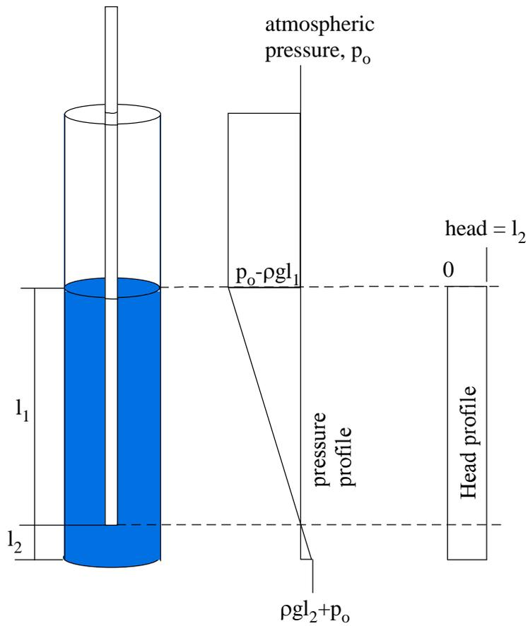
While the water is above the bottom of the tube, the head in the Cylinder is constant (at a value of  $l_2$ ) because the pressure at the bottom of the tube remains atmospheric.
