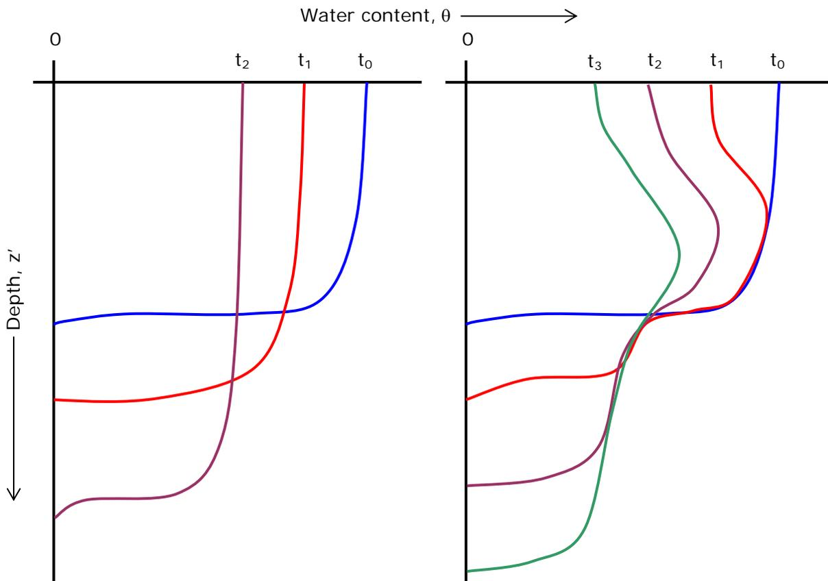
Profiles show a typical water distribution after deep soil infiltration in the absence of evaporation.  $t_0$  is defined as the time when redistribution begins.
