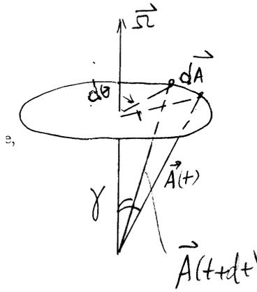
Figure 7.1.1: Vector  $\vec{A}(t)$  rotating at the angular velocity  $\vec{\Omega}$ .
