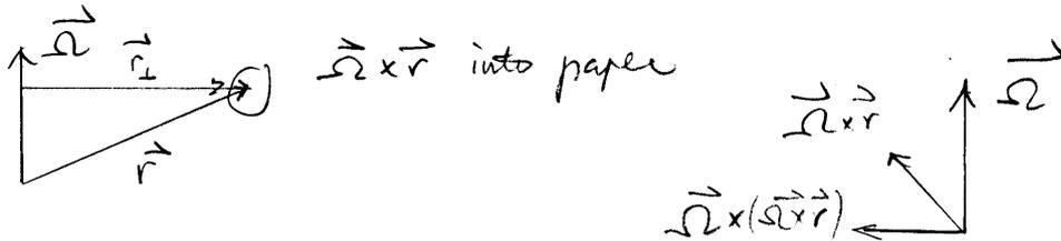
Figure 7.1.2: Coriolis force, position vector and angular velocity
