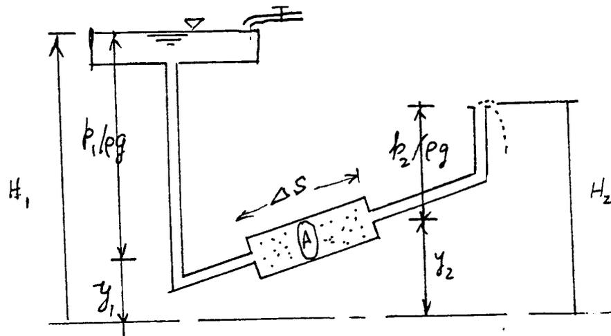
Figure 6.1.1: Darcy's experiment for seepage flow
