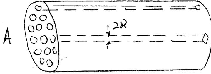
Figure 6.1.2: A one dimensional model of porous medium
