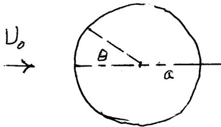
Figure 3.8.3: Definition of coordinates for a circular cylinder.
