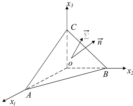
Figure 1.4.2: Stress components on any surface element
