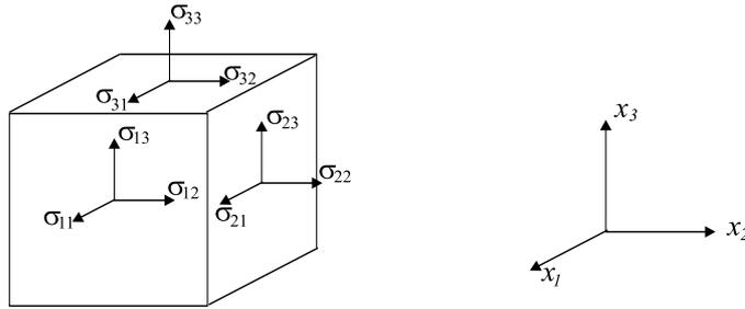
Figure 1.4.1: Stress components on a fluid element
