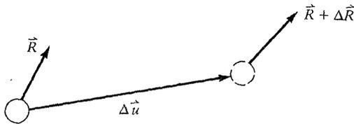
Fig. 7-3. Virtual displacement of a single mass particle.
