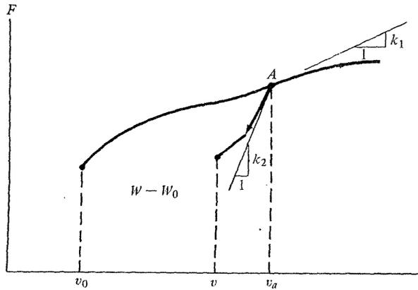
Fig. 7-2. Work integral for direction-dependent force.
