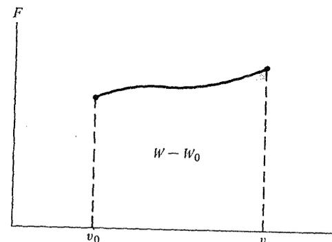
Fig. 7-1. Work integral for the one-dimensional force-displacement relation.
