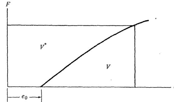
Fig. 7-5. Graphical representation of strain energy and complementary energy.
