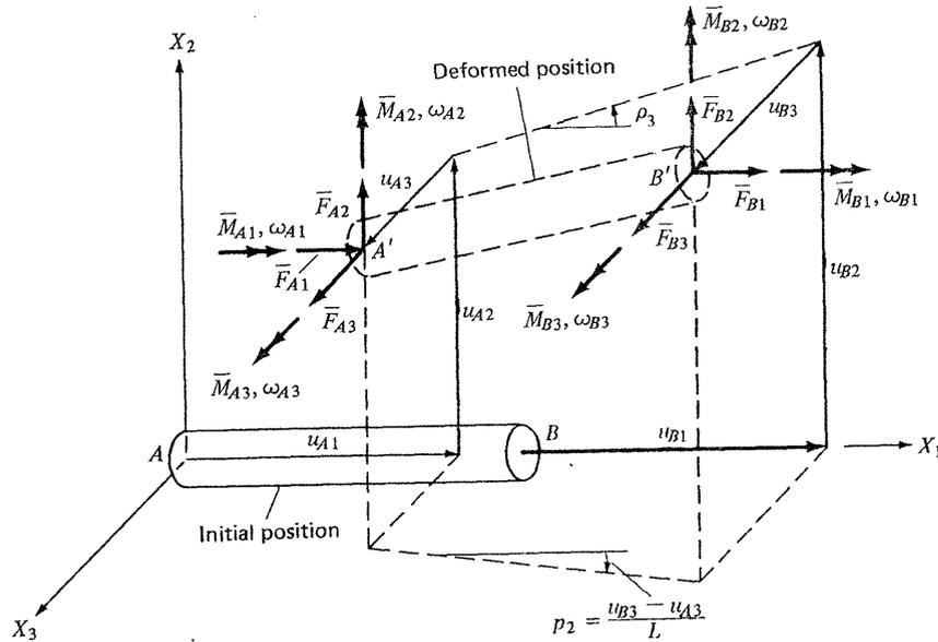
Note: The centroidal axis coincides with  $X_1$ .  $X_2$  and  $X_3$  are principal inertia directions.
