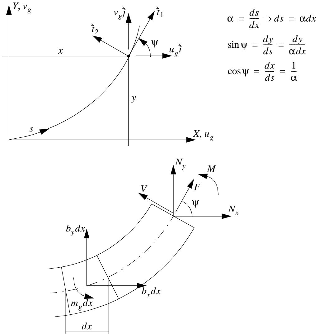
The above figure defines the “cartesian” notation. The distributed loading ( $b_x, b_y, m_g$ ) is defined with respect to the  $x$  and  $y$  directions and the loading per unit projected length ( $dx$ ). Similarly, the displacement components ( $u_g, v_g$ ) are referred to the cartesian global reference directions.
