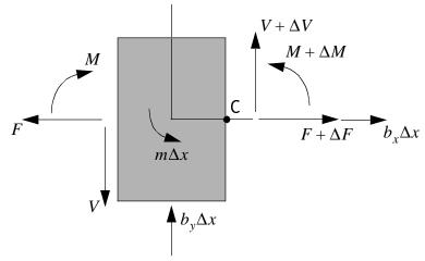
Consider the rate of change of the internal force quantities over an interval  $\Delta x$
