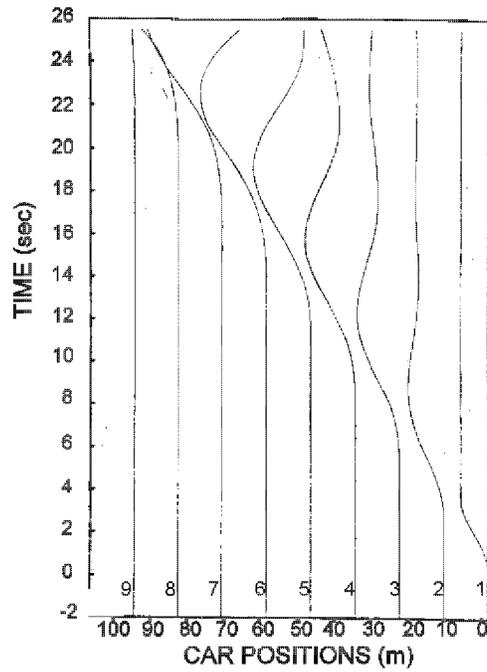
Note: Diagram illustrates the linear car following equation, eq. 4.23, where  $C=0.80$ .
