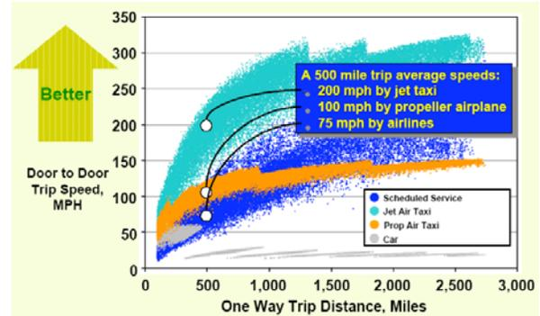
Figure 3: Door to door trip speed for various mode of transportation (SATS) [7].
