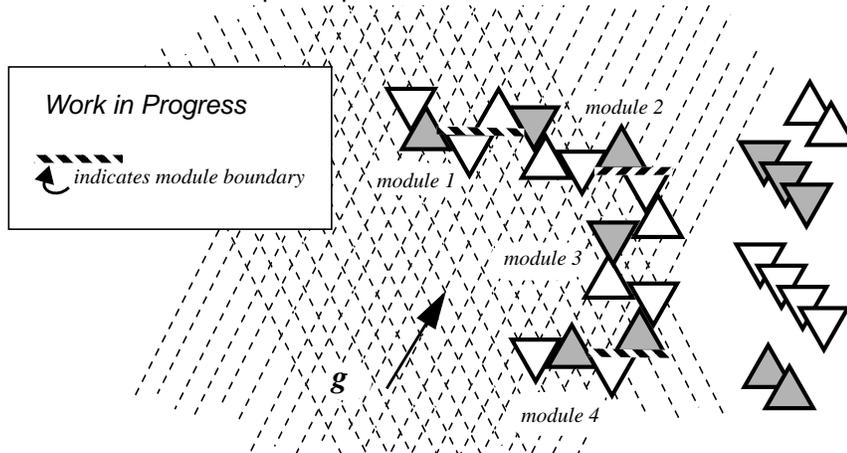
The individual modules into which a given structure will be decomposed and constructed at the factory are easy to identify, because the boundaries between them are defined by the orientation of the joints relative to gravity. To an earthly eye, any intersection of two deltas that runs left to right, across the page, is a module boundary. The figure shows how this works. The design has 3 such joints, and therefore 4 modules.
