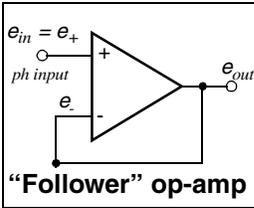
**Note** too that if we let  $R_1$  get very large (e.g., open the leg to ground) and let  $R_2$  get vanishingly small (short circuit pin 2 to the output pin 6), then we have the circuit you used in the first part of the course as a “buffer” or “follower” - an instrumentation amplifier which did not “load down” your ph sensor (recall rule 2) and supplied as much current as needed at its output *with a gain of  $G = 1$* .
