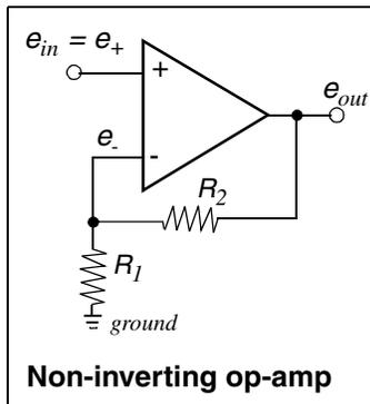
As an example of a single input application, consider the “non-inverting amplifier” shown at the left. First some rules of behavior of our black box. Quoting *The Art of Electronics*:
