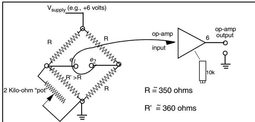
If available, use two voltmeters to measure both the input voltage to the op-amp  $e_1 - e_2$ , and the output voltage of the op-amp, pin 6 to ground. First, short out the input, connecting  $e_1$  and  $e_2$  using a short jumper wire. Then, adjust the 10 Kohm trim pot until the output of the op-amp is zero, i.e., within a few millivolts of zero. (Zero does not exist in the material world).
