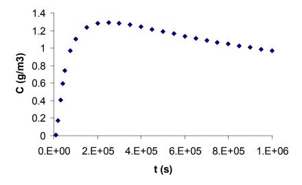
From this plot, we can see that the maximum concentration at the house is approximately **1.3 gm**<sup>-3</sup> (when  $t \approx 2.4 \times 10^5 \text{ s} = 67 \text{ hrs}$ )
