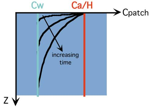
**Figure 8.** Diffusion of mass into a new patch brought to the surface at  $t = 0$ . Before patch arrives at surface ( $t < 0$ ),  $C = C_w$  throughout the patch. For  $t \geq 0$  the concentration at the patch-air interface ( $z = 0$ ) is at equilibrium with the air,  $Ca/H$ .
