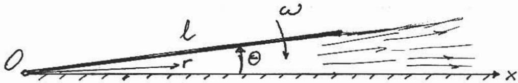
A plate of length  $l$  (very long into paper, so problem may be treated as 2-D) rotates around a pivot point,  $O$ , at an angular velocity  $\omega$  [rad/s] forcing the plate down towards a horizontal surface. The angle between the rotating plate and the surface,  $\theta$ , is decreasing with time and water filling the gap is being squeezed out.  $\theta \ll 1$  [rad] so  $\sin \theta = \tan \theta = \theta$ ,  $\cos \theta = 1$ .
