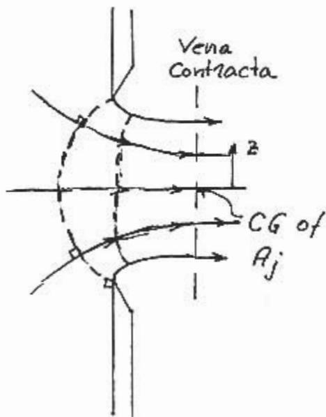
In vicinity of the hole streamlines are curved, so pressure is not hydrostatic across the area of the hole in the bucket wall. However, after the flow has turned the corner the streamlines become straight (and parallel) at the so-called "vena contracta". Our control volume is chosen to cut across the jet at its "vena contracta".
